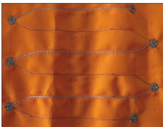
Fig. 6. Optimised J-type F-TEG with Stainless steel: Constantan threads ratio 3:1 Electric circuit Ohmic resistance: 300 \Omega
