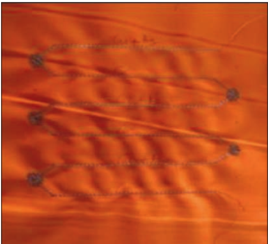
Fig. 3. F-TEG type T Pairs of legs of Constantan and Copper threads Junctions consolidated by Silver threads Electric circuit Ohmic resistance: 55 Ω
